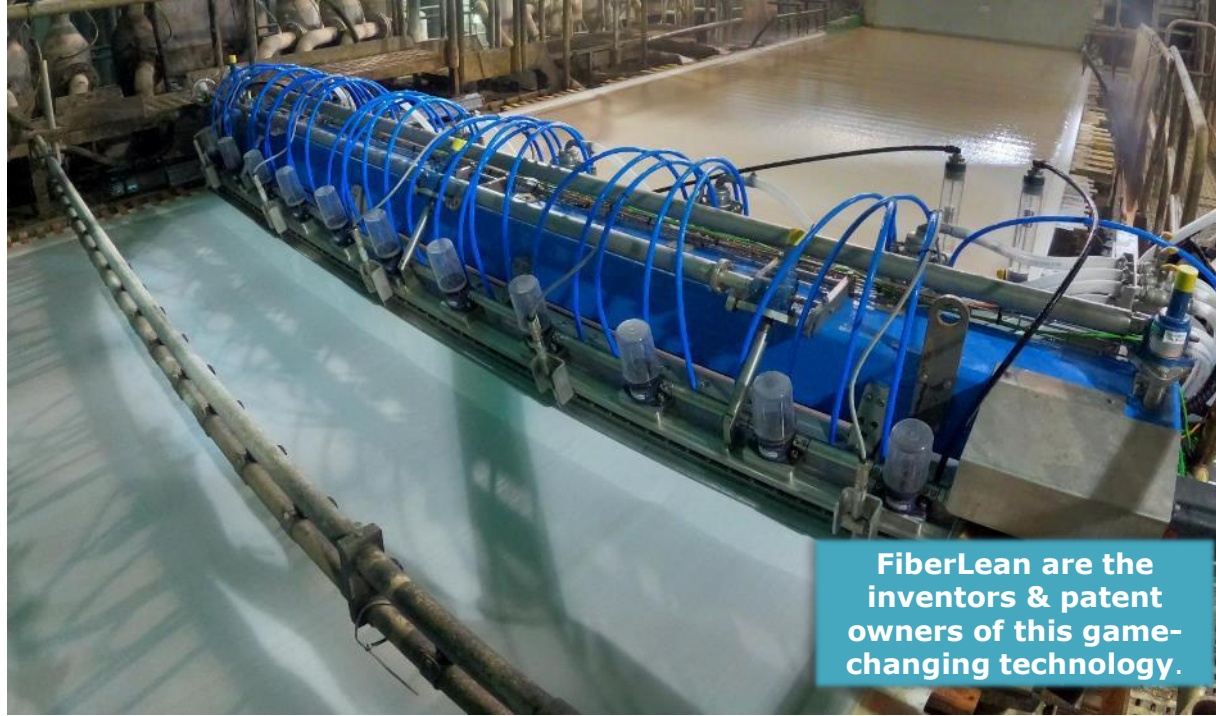
Image: 3-meter wide FiberLean on Top (FLoT) applicator operating on a paper machine running at 500 m/min
